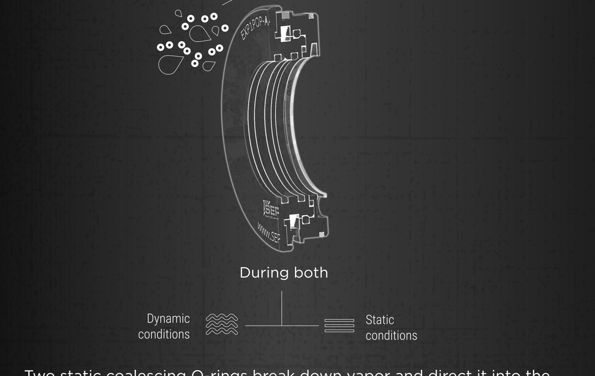
Two static coalescing O-rings break down vapor and direct it into the expeller chamber. The condensate chamber becomes a trap for moisture. During dynamic operation, centrifugal force adds energy to contaminants and expels them from the internal environment.
