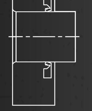
A lip seal's ability to block contaminants degrades with operation. As the seals wear, contamination is introduced and increases as wear continues.
